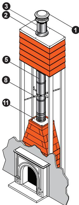
Prefabricated Masonry Fireplace Kit with Metal Chimney
