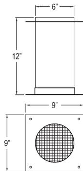
Allows required ventilation air into chase. Screen keeps rodents out.
