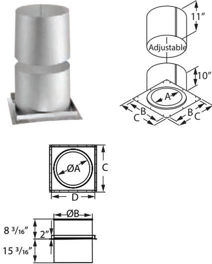
Use in ceiling/floor penetrations other than those that include the ceiling support. Fits on underside of ceiling and adjusts to cover framing.
