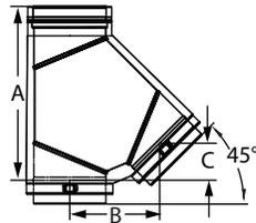
Use in place of any DuraVent tee for a 45° angle instead of 90°; can be used as a manifold connection to gang multiple boilers into a common vent.
