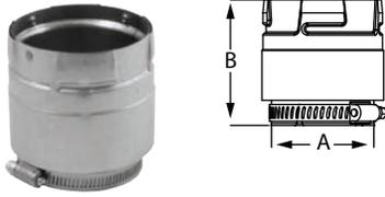
Use to attach to appliance outlet allowing for easy pipe connection. Features an adjustable hose clamp and gasket to form a tight seal. The hose clamp can be loosened and tightened as needed to disconnect and connect the vent to the appliance.
