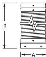
Use through damper and smoke shelf area. Use with DuraLiner Insulation Kit (ProMesh and ProFoil), where flex extends into clay liner, for zero-clearance applications. Built from 1-ply construction, .005" 304 stainless steel.
