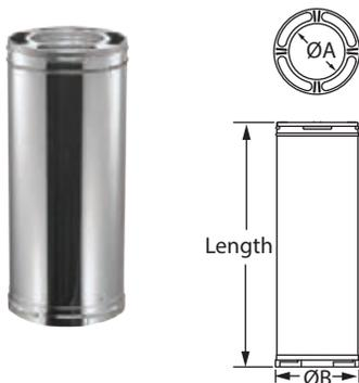
Designed for appliances tested and listed for use with wood stoves, fireplaces, furnaces, boilers, stoves, ranges, water heaters, or other appliances fueled by wood, oil, coal, or gas. 6", 9", and 12" chimney pipe has 1" insulation blanket; 24", 36" chimney pipe has 1/2" insulation. To calculate the installed length of DuraPlus chimney pipe, subtract 1 1/2" from each length of chimney pipe.
