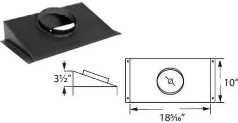
Use to connect inserts with either rectangular or round flue collars to 6" or 8" liners. Made from 11 gauge carbon steel.
