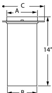
Used to adapt DuraBlack pipe to 6" - 8" Ceiling Support Box, including DuraTech, DuraPlus, and DuraTech Premium systems. The Slip connector can also be added to 6" - 8" DuraTech finishing collar. Adds 3"-13" of length to rigid pipe. Provides a strong mechanical connection.
