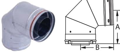
Use to go from horizontal to vertical runs or vertical to horizontal runs. Use to turn vent 90°. Sloped at 88° to direct condensate back to the appliance.
