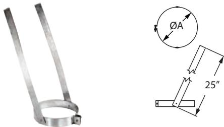
Use to prevent excessive weight on the elbows by supporting the weight of the chimney. Required to be installed between two elbows in offset installations. Multiple elbow straps may be required for offset installations. Refer to installation instructions.
