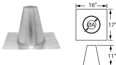
Use to weather proof the penetration of vent pipe through the roof. Storm Collar required. Select roof flashing based on pitch of roof. Use on flat roofs, chase enclosures, or masonry chimney. Made of galvalume.
