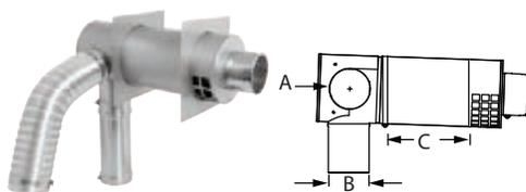
Use for through-the-wall termination with direct vent wall mounted gas appliances. an adjustable right and left hand air intake snout and accommodates wall thickness of 10" - 18". Check installation instructions for restrictions on horizontal termination, such as minimum distance from windows and doors.
