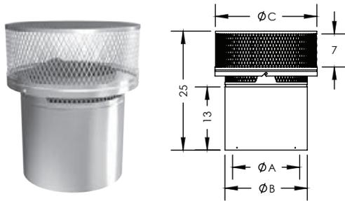
Use to terminate chimney system. Required on all installations. Slides over previous section of DuraChimney II pipe to allow for chimney height adjustment. Includes Spark Arrestor.
