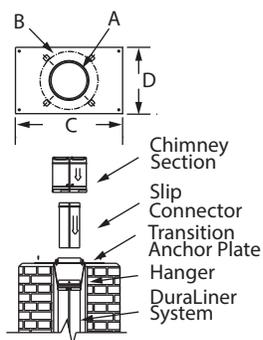
Use with Slip Connector and Hanger in chimney restoration to connect DuraLiner pipe to DuraTech, DuraPlus, or DuraTech Premium Chimney. Painted black. Pricing for Transition Anchor Plates are listed under DuraTech, DuraPlus, and DuraTech Premium.
