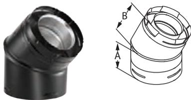
Use to offset obstructions as needed. Fully unitized, twist-lock construction. Elbows swivel, allowing the lock to remain fully engaged while aligning to the desired direction. The angle will remain fixed at 45°.
