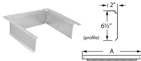
Required at top of chase enclosure or where chimney passes through the roof. Roof Radiation Shield is not required if chimney is unenclosed in the attic. Four plates (included) make up one shield. Three of the four plates shown.
