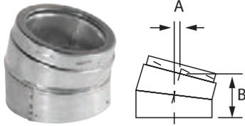
Use to offset chimney around obstacles such as a joist or truss. A maximum of two offsets (4 elbows) is permitted. Each elbow is sold individually.
