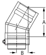
Offsets obstructions as needed. Allows for better condensate management and less back pressure.
