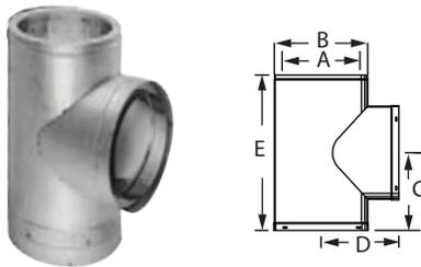
Use for through-the-wall installations. Includes removable Tee Cap for easy chimney cleaning or inspection. Wall Straps, a Wall Thimble, and an Adjustable Tee Support Bracket must be installed with the Tee as directed. Available in stainless steel or with a galvalume outer wall and stainless steel inner wall. 18"-24" Tee is not UL listed. See installation instructions for proper location and installation of Tee.
