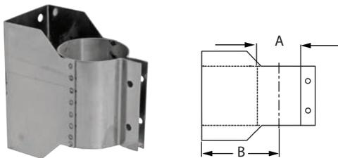
Use to support vent pipe or tee sections. Provides proper clearance to combustibles. When installing FasNSeal W2 with this component use 1" larger diameter, (e.g. 10" vent system, use 11" size).
