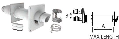
Use for concentric horizontal terminations. Includes 2 appliance adapters, white wall plate, white firestop, and co-linear adapter. White Termination with Bird Guard Screen. UV resistant. Inner plate is 8 5/8" (220mm) square, outer plate is 9 7/16" (240mm) square for all flue sizes. Includes 2 Locking Bands and two Adapter Connector clamps. Adapters included to transition from PVC appliance outlet to twin pipe PolyPro.
