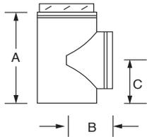
Located at the base of the chimney, it provides the horizontal connection to the appliance. It is recommended for installations where a connector must pass through an exterior wall because its insulation prevents the cooling of chimney gases. An insulated tee cap is included.
