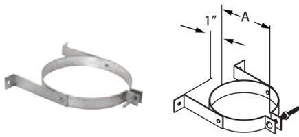
Use to support vent pipe. Provides 1" clearance. Recommend installing Wall Straps at 4-foot intervals on vertical runs.
