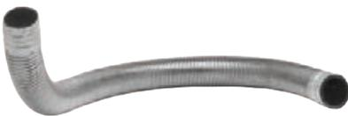
Use for offsetting rigid pipe around smoke shelf in masonry chimney only. Allows for offsets with biofuel appliances. Female and male ends twist-lock. Female end swivels for easy alignment. 5' flex section. Not for use in attic or wall spaces.
