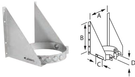
Use to support the chimney on a vertical wall. The triangular plates allow a 2" to 4" lateral adjustment of the support to the vertical surface. This support can also be used as a wall support above the insulated tee or as a support for an offset elbow. Refer to chart for loadbearing capacity. In shorter chimney stack applications, the Re-Support can also be used in place of a Tee Support. Universal design works with 6", 7", or 8" pipe diameters.
