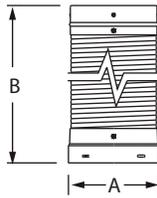
Use through damper and smoke shelf area. Built-in fittings. Use with DuraLiner Insulation Kit (ProMesh and ProFoil), where flex extends into clay liner, for zero-clearance applications. Round-to-Round Flex pipe built from .016", 304 stainless steel, 4-ply construction.
