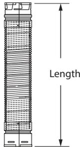
Use as a connector system to replace rigid gas vent with a flexible section. DuraConnect II can be used when Type B gas vent double-wall connector is required. Not to be enclosed and cannot penetrate through walls, floors, or ceilings. Twist-lock connectors on each end.
