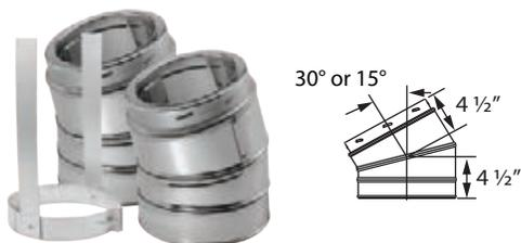
Elbow Kit includes: 2 Elbows and 1 Elbow Strap. Use for offsets around obstructions such as rafters, ridgepoles, or joists. May have two pairs of elbows, if needed. Offsets greater than 30° are not permitted in accordance to UL 103 standards. Elbows swivel 360° at base (angles are not adjustable). A pair of elbows is required to return an offset chimney back to vertical. Available in stainless steel (5"-8" SS) or galvalume (6"-8" GA) outer wall.
