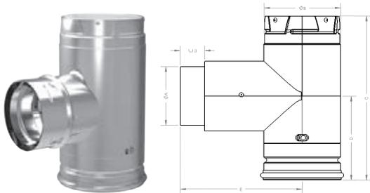
Attaches 3" pipe to branch and 4" pipe to body. Use for a 90° offset. Branch swivels for alignment. One piece unit incorporates removable twist-lock Clean-Out Tee Cap.
