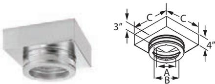
Supports chimney pipe and provides a positive connection between support box and chimney with a built-in twist-lock. Designed for installation in flat ceilings only. Supports up to 60' of DuraTech Chimney. Use adapter to attach DVL or DuraBlack to the support box. A 2" wide trim collar is included. Not painted, but can be painted with high temperature paint. (For adapters see DVL/DuraBlack section).
