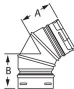
Offsets obstructions as needed. Elbows swivel 360° at base. 45°/60° Elbow is adjustable from 0° to 60°. Elbows must be supported when installed.
