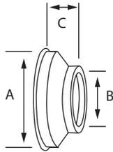
Use to conceal the protrusion of the insulated length (5") inside the dwelling. A flue extension must be used to ensure a perfect connection between the chimney and the double-wall black connector.
