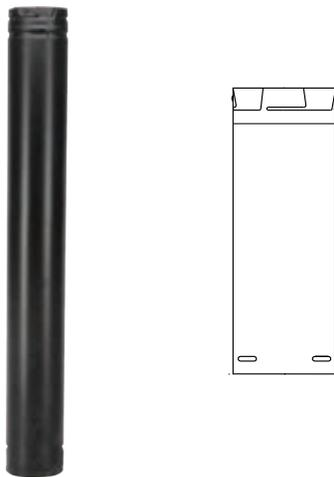
Features fully unitized, twist-lock construction in 3" and 4" diameters. Listed at 1" clearance to combustibles in the USA and Canada. It can be used in both vertical and horizontal installations. Stainless steel welded seam inner wall, combined with a galvalume welded seam outer wall. Pipe OD is diameter plus 5/8". Galvalume or painted black outer finish. 12" length available with stainless steel outer (SS). To calculate installed length, subtract 1 1/2" from each length of pipe.
