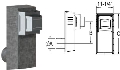
Use for horizontal through-the-wall termination when a vertical rise is desired in the system to meet appliance manufacturer recommended minimum heights. Do not enclose in the wall or install below grade. Provides improved performance in high wind conditions. Features an adjustable air intake and interchangeable shroud (shroud is included and required for all installations). Check with appliance manufacturer for approval and air throttle setting. Patent Pending.
