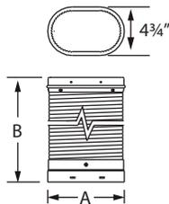
Use through damper and smoke shelf area. Built-in fittings. Use to connect from oval stove outlet to round DuraLiner. Use with DuraLiner Insulation Kit (ProMesh and ProFoil), where flex extends into clay liner, for zero clearance applications. Oval-to-Oval Flex pipe built from .016", 304 stainless steel, 4-ply construction.
