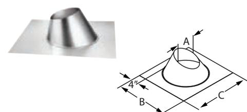
Use with metal or tile roofs. Available in sizes 4"x 6 5/8" and 5"x 8", in 0/12-6/12 (shown) and 7/12-12/12 styles. Made of malleable dead soft aluminum. Refer to roof flashings tables (previous page) for dimensions.
