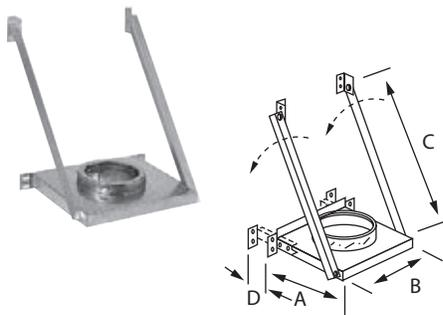
Supports the chimney at the base of the installation, functioning similarly to the tee support but with an adjustable base to provide additional wall clearance as needed. The tee support must be installed with the insulated tee cap included with the insulated tee. Coupler included.
