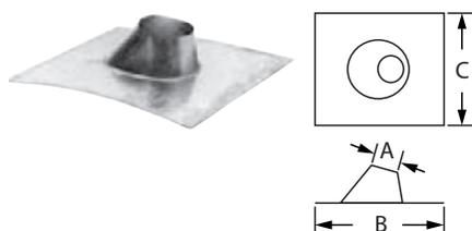
Use to weather proof the penetration of vent pipe through the roof. Fits up to 7/12 roof pitch. Storm Collar required. Made of malleable dead soft aluminum.
