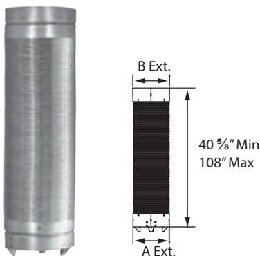
The Flexible Shield is used in much the same fashion as the Telescopic Rigid Shield (TRS) but will be required where offset elbows are involved. Includes stand-off spacers. Must be installed as per instructions.
