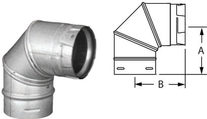
Offsets obstructions as needed. Elbows swivel 360° at base. Angle not adjustable.
