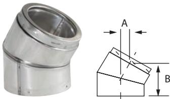
Use to offset chimney around obstacles such as a joist or truss. A maximum of two offsets (4 elbows) is permitted. Each elbow is sold individually.
