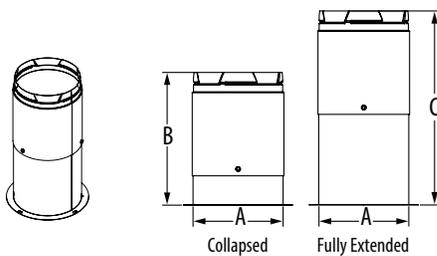
Adjustable Adapter with flange for galvanized outer jacket. Flange attaches to appliance cabinet with supplied screws. To calculate installed length, subtract 1 1/2" for each joint.
