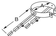
Designed to stabilize a chimney extending from 60" to 115" beyond the roof, or when a chimney is exposed to high winds. This part is supplied with tightening collar and adjustable legs.
