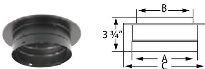
Use to connect from double-wall DVL to DuraTech, DuraPlus, DuraTech Premium, and DuraLiner for a through-the-wall or ceiling support installation. Required for proper connection. Provides a strong mechanical connection. Painted black. Adapter will work with all 6"-8" DuraPlus, 6"-8" DuraTech Premium, and 7"-8" DuraTech installations. Adapter will work with 5"-6" DuraTech Ceiling Support Box installations only.
