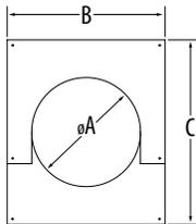
Use when penetrating walls or floor levels. Two piece design for easier installation.
