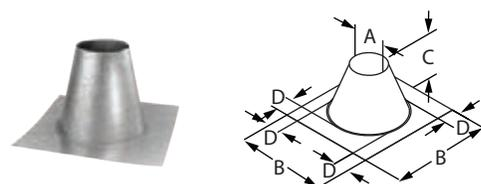
Use to weather proof the penetration of vent pipe through the roof. Storm Collar required. Use on flat roofs, chase enclosures, or masonry chimney. Made of galvalume.
