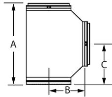
Use to transition from horizontal to vertical with improved flue gas flow with angled gradual transitions. Can also be used as a manifold connection to gang boilers into a common vent. Completely welded inner walls.
