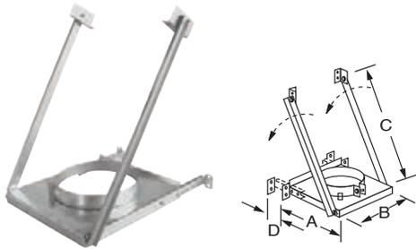
This part supports the chimney at the base of the installation or along a wall or other vertical surface serving as an intermediate support. It comes with a tightening collar that locks around the chimney and is secured by two self-tapping screws (included).
