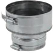
Use to connect 4" diameter Ventinox flex to a 3" diameter pellet insert.
