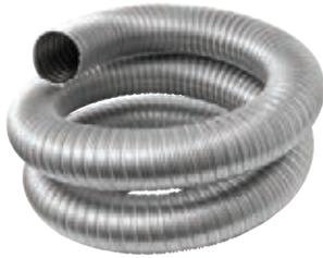
Use to vent Category II,III and IV gas burning appliances. Listed to UL 1738. Can only be used in vertical or near vertical runs. **Custom lengths are available for 3"-12" diameters.** Minimum length of 10' for custom orders. Maximum length of 50' for 3" - 9" diameter custom orders and 25' for 10" and 12" diameter custom orders. Must be ordered in 10' increments. Use with FasNSeal components only.
