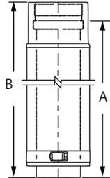
Use to add variable length to your straight length of FasNSeal pipe. Adds 2"-14" of length. Requires at least 4" overlap for a secure connection.
