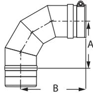
Use to go from horizontal to vertical runs or vertical to horizontal runs. Use to turn vent 90°.
