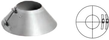
Use to create a weather tight seal between the pipe and flashing. When installing FasNSeal W2 with this component use 1" larger diameter, (e.g. 10" vent system, use 11" size).
