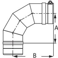
Use to transition from a vertical to a horizontal run. Stabilizes a 2° pitch towards the condensate drain for good condensate management.
