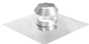
Used to support the liner from the chimney allowing space for thermal expansion. Made of stainless steel (type 304); it includes a support collar locking around the flue, and a storm collar to ensure a watertight seal.
