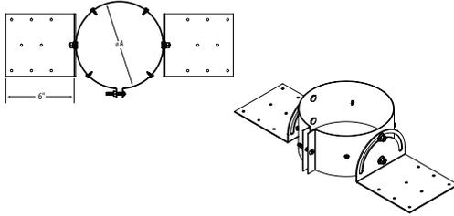
Used to support galvanized outer jacket and PolyPro vent within at the roof level. Adjustable to different roof pitches. Ideal for cathedral ceilings.
