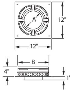
Use to adapt on a zero-clearance fireplace when using DuraPlus directly off the unit. Starter Section built in.
