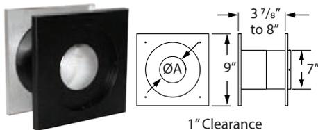
Use for through-the-wall installations. Fits between standard wall studs. Comes with an insulation ring to reduce air infiltration where the pipe slips through the thimble.
