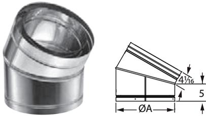
Use elbows to offset obstructions such as rafters, ridgepoles, or joists. 10"-16" DuraChimney II may have two pair of elbows, if needed. Offsets greater than 30° are not allowed. Elbows are not adjustable.
