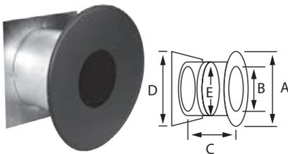
Designed to protect surrounding combustible materials when a chimney passes through a wall. Adjustable to permit use with walls from 7" to 12 1/2" thick. Insulated to help prevent cold air intrusion.
