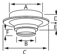
Use to support the chimney at a ceiling. Designed to connect to both double-wall and single-wall stove pipe. It is enhanced by a decorative black finish. Fits even narrow joist spaces with a 12" diameter for 6" chimney. Must be attached to a frame built from the joists (refer to loadbearing capacity and size of openings chart). Removable trim collar is great for retrofit and new construction. Coupler included.
