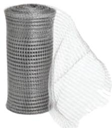
Use to protect the ProFoil during installation. 304 stainless steel mesh slides over insulated liner. Shrinks to fit liner when pulled length-wise.
