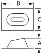
Use with metal or tile roofs. Available in Adjustable Roof Flashing style (0/12-6/12). Made of dead soft aluminum. Refer to Roof Flashing tables for dimensions.
