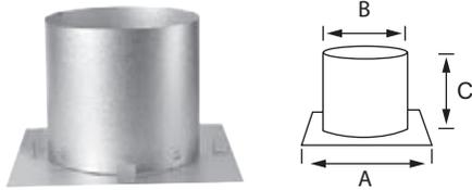
Use to protect combustible materials when the chimney passes through a floor or an intermediate ceiling. It ensures a 2" safety clearance between the chimney's outer casing and surrounding combustibles. When passing through a ceiling, it must be installed from the underside of the ceiling. Required in some jurisdictions in replacement of the firestop.
