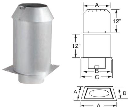
Also referred to as an insulation shield, this has the same features as the two-piece insulated attic radiation shield but its height is adjustable from 12" to 22". Insulated to prevent cold air intrusion. Storm collar included.
