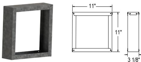
Use as a heat shield on structures with vinyl siding, or other temperature sensitive materials, to help prevent warping and or melting of the material. Use only on horizontal terminations and on any irregular surfaced siding (ie: ship lag siding, shake shingle siding) so cap is not imbedded in the siding. Sized for Sconce Cap, Round Horizontal Cap and H2 Horizontal Cap only. Factory assembled. Use for 4"x 6 5/8" and 5"x 8" diameters.
