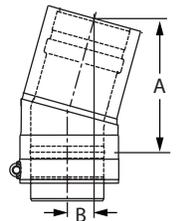
Offsets obstructions as needed. Allows for better condensate management and less back pressure.
