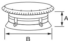
Attached to the top of the chimney, it effectively prevents rain, snow and leaves from entering the opening.
