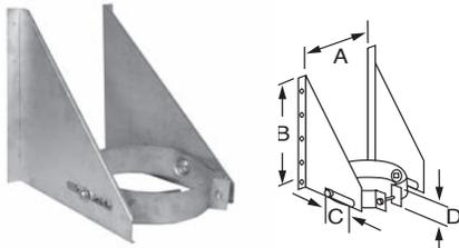
This part is designed to support the chimney on a vertical wall. The triangular plates allow a 2" to 6" lateral adjustment of the support to the vertical surface. When used as a tee support, it lends itself to the addition of a Twist-Lock insulated tee cap.
