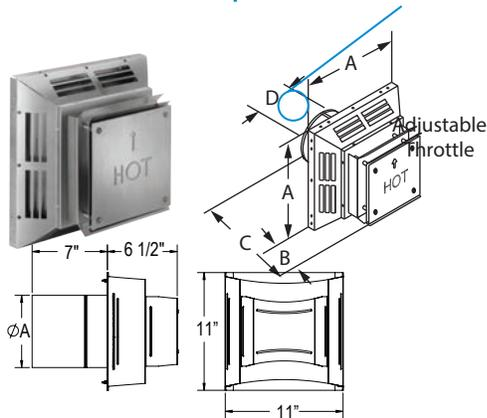
Use for standard and high-wind through-the-wall termination. Check installation instructions for restrictions on horizontal cap terminations, such as minimum distance from windows and doors. Available in aluminum, stainless steel (S), and copper (C).
