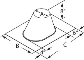
Use with metal or tile roofs. Available in sizes 6" and 8" in large base 0/12-6/12 (shown) and 7/12-12/12 styles. Made of dead soft aluminum. Refer to Roof Flashing table for dimensions.
