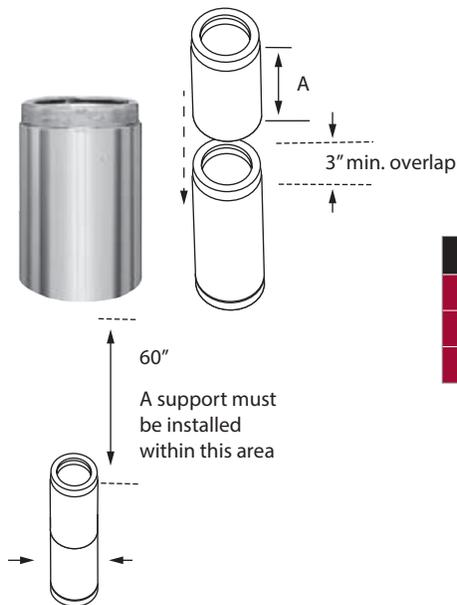
Used in combination with straight insulated lengths, the adjustable length makes it possible to fit a DuraTech Canada length perfectly.
