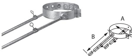
Stabilizes a chimney extending from 60" to 115" beyond the roof, or when a chimney is exposed to high winds. This part is supplied with tightening collar and adjustable legs. Universal design permits use with 6", 7", and 8" diameter pipe. Note: Not intended to provide protection against sliding ice and snow.
