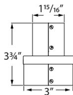
Use to increase an insert's 2" air inlet to connect to 3" aluminum flex.
