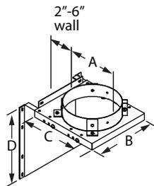
Use as wall support for chimney system. Use of straps is optional. Supports up to 50' of DuraTech Chimney without straps, and 70' of DuraTech Chimney with straps. Attaches to chimney pipe. Can be installed above or below the Tee. If installed below the Tee, a short section of pipe is required. Adjustable base provides 2" to 6" clearance to wall.
