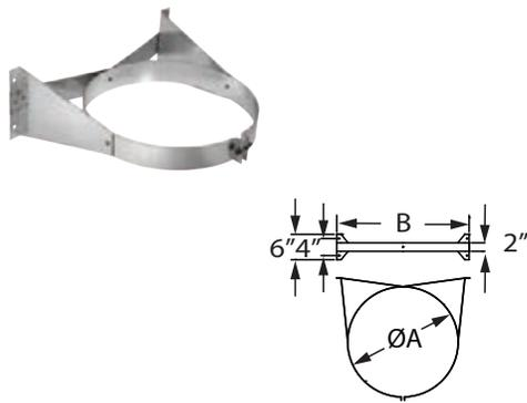
Use in interior or exterior installations to add lateral support to the chimney. Assures a 2" clearance to combustible walls. Required every 4'.
