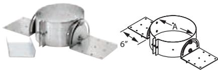
Designed to support the DuraTech Chimney and allows the chimney to pass through the roof and extend down the ceiling. Ideal for cathedral ceilings and free-standing appliance installations. Supports a maximum total chimney length of 45' above and 20' chimney below Roof Support. Adjustable to different roof pitches.
