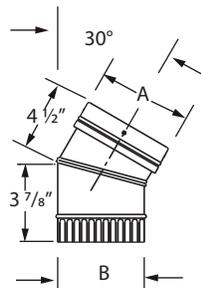
Use as a insert connector to DuraLiner. Features built-in fittings for easy connection to DuraLiner. Elbows are single-wall.
