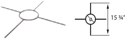
Use to support PolyPro Flex from top of masonry chimney or chase.
