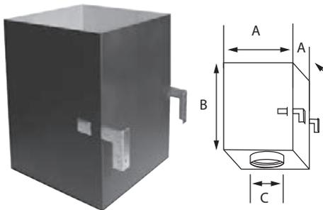
This specialty support can be used where space is limited such as shallow attics. Attachment arms provide up to 2 1/2" of play to allow for box alignment. Includes Coupler. Works with either double-wall or single-wall stove pipe. Refer to installation instructions for further details.
