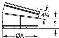
Use elbows to offset obstructions such as rafters, ridgepoles, or joists. 10"-16" DuraChimney II may have two pair of elbows, if needed. Offsets greater than 30° are not allowed. Elbows are not adjustable.
