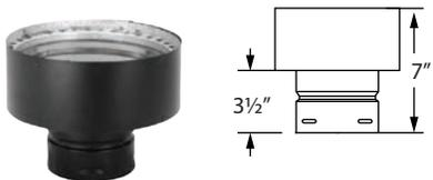
Use to transition between PelletVent Pro to existing chimney such as DuraTech, DuraPlus or DuraTech Premium. Requires a DVL/ DuraBlack Chimney Adapter to fasten into support box or wall thimble, for 6", use adapter 6DVL-ADC or 6DVL-ADT, for 8", use adapter 8DVL-ADC or 8DVL-ADT.
