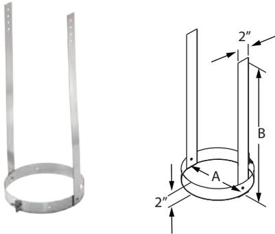
Use to prevent excessive weight on the elbows by supporting the weight of the chimney. Required to be installed between two elbows in offset installations. Multiple elbow straps may be required for offset installations. Refer to installation instructions.
