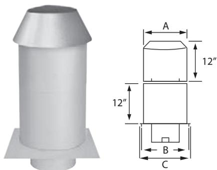
Protects combustible materials when a chimney passes through an attic. Height is adjustable from 12" to 22". It is imperative that it be installed overside from the attic. Its collar keeps insulation from seeping between the outer casing and the firestop. It also maintains a 2" clearance from combustible materials. A firestop (FS) is not needed when a support is used directly below. Insulated to prevent cold air intrusion.
