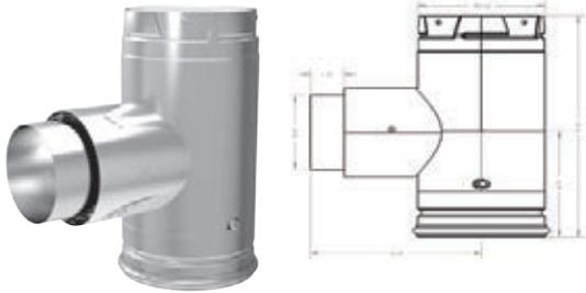
Use for a 90° offset. Attaches directly to appliance as an adapter. Converts a 3" appliance to a 4" PelletVent Pro system. One piece unit incorporates removable twist-lock Clean-Out Tee Cap.
