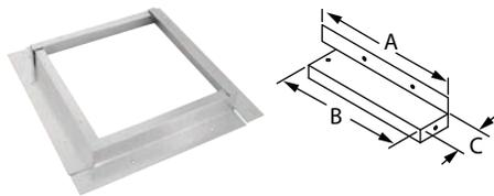
Prevents water intrusion into stucco-sided homes. Allows the installer to apply siding material (ie: stucco, brick, etc) over the flanges up to the sides of the flashing for a water-tight seal. Kit includes 4-pieces; sized for 4" x 6 5/8" Sconce Cap, Round Horizontal Cap and H2 Horizontal Cap only. Also available in stainless steel (S). Use for 4" x 6 5/8" and 5" x 8" diameters.
