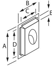
Designed for use when the chimney passes through a wall at an angle. Insulated to prevent cold air intrusion.
