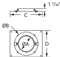
Use Transition Anchor Plate with DuraPlus when extending or converting from DuraLiner to DuraPlus in chimney restoration. Use with DuraLiner Slip Connector and Hanger. (See DuraLiner section.)
