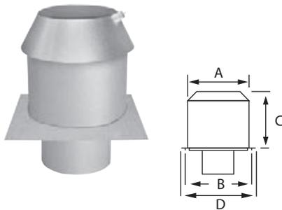
Protects combustible materials when a chimney passes through an attic. It is imperative that it be installed overside from the attic. Its collar keeps insulation from seeping between the outer casing and the firestop. It also maintains a 2" clearance from combustible materials. A firestop is not needed when a support is used directly below. Insulated to prevent cold air intrusion.
