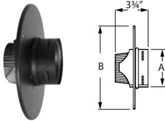
Use to connect PelletVent Pro rigid pipe to a masonry chimney with stainless steel flexible relining. Female end swivels to allow ease of connection.
