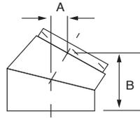
Allows the 45° offset of a chimney. Designed to bypass an obstacle, such as a joist. A maximum of two offsets (4 elbows) is allowed. The chimney's angle of inclination must not deviate more than 45° from the vertical position.
