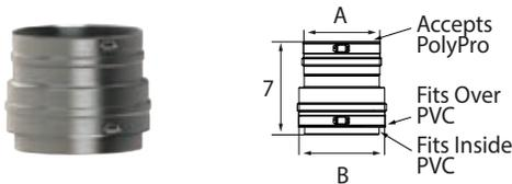
Use to directly connect PolyPro to a male PVC Pipe appliance outlet. Seals on the O.D. of the PVC pipe and has a clamp. No adapter connector and/or Locking Band required.
