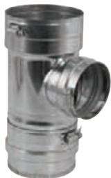
Used to connect flex to pellet insert. Use as a 90° transition between liner and connector pipe at the wall thimble or rear flue outlet of a pellet appliance. Transition from 3" PelletVent to 4" Ventinox Chimney Liner. Tee is 9" tall. Comes with Clean-Out Cap.
