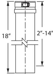
Use to add length to straight length of FasNSeal pipe. Adds 2"-14" of length. Requires at least 4" overlap for a secure connection.
