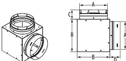
Adjustable Adapter with flange for galvanized outer jacket. Flange attaches to appliance cabinet with supplied screws. To calculate installed length, subtract 1 1/2" for each joint. Includes metal support ring.
