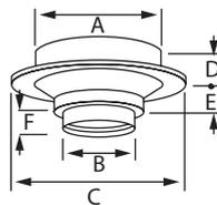
Use to support the chimney at the ceiling. Includes coupler to work with either double-wall or single-wall stove pipe. Allows 6" pipe to fit within a minimum 12" x 12" framed opening. Black finish.
