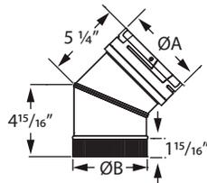
Use to offset obstructions as needed. Use as a insert connector to DuraLiner. Features built-in fittings for easy connection to DuraLiner. Elbows are single-wall.
