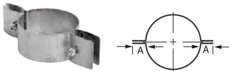
Use to support vertical and horizontal runs. Recommended every 10' in the vertical run. Use additional Support Clamps as needed. When installing FasNSeal W2 with this component use 1" larger diameter, (e.g. 10" vent system, use 11" size).
