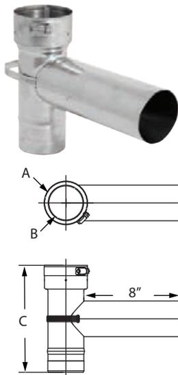
Use as a 90° transition between liner and connector pipe at the wall thimble or rear flue outlet of a heater. Removable Snout with internal draw band allows for easier, through the wall thimble installation. 5 1/2" diameter has a 6" branch.
