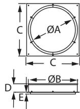
Use as a starter section for DuraTech. Bolts directly to masonry fireplace outlet.
