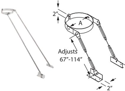
Use to support the chimney when it extends more than 5' above the roof. Provides stability to chimney against wind and snow. Mounting brackets and adjustable tubing included.
