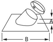
Use to accommodate chimney installation on sloped roof. Choose from 3 different pitches in standard or aluminum malleable versions. Storm collar is included.
