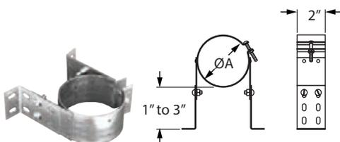
Use to support vent pipe or tee sections. Adjusts to provide 1"- 3" clearance.
