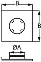
Encloses the top of a chase while providing a ventilation air passage from the chase. UL Listed. Includes spacer clips. Storm collar not included. Made of galvalume.
