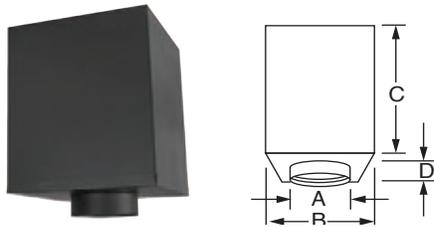
Use with flat, vaulted or cathedral ceilings. Certified to reduce clearance to combustibles from the usual 2" (per side) down to a 1" (per side) for all diameters. This allows for a smaller hole to be cut in the ceiling. Can connect to both double-wall stove pipe or single-wall stove pipe with included adapter. Functions as both an Attic Insulation Shield and Finishing Support. An adjustable black finish trim insulation pad and collar are included.
