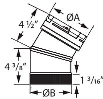
Use to offset obstructions as needed. Use as a insert connector to DuraLiner. Built-in fittings for connection to DuraLiner. Elbows are single-wall.
