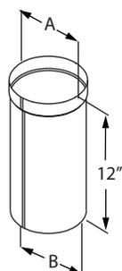
Connects to the oval flue outlet of the appliance. Must be field ovalized.
