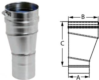
Use to transition to a larger diameter pipe. Prevents condensate puddling when used on horizontal runs. Aids in reducing formation of condensates. **Additional sizes available up to a maximum of 10" diameter change.**
