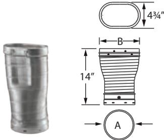
Use to connect a round stove outlet to oval DuraLiner. Use with DuraLiner Insulation Kit (ProMesh and ProFoil), where flex extends into clay liner, for zero-clearance applications. Built from 304 stainless steel.
