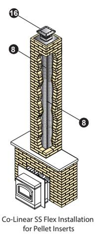
Co-Linear SS Flex Installation for Pellet Inserts
