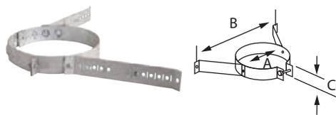
Use on an interior or exterior wall. Provides stability for the chimney while also maintaining required clearances to combustible surfaces. Wall Straps are recommended at 8' intervals. Can be adjusted to permit standoff distance of 2" up to 6". Universal design can be used on 6", 7", and 8" pipe diameters.
