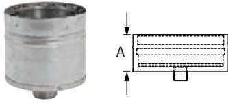
Use to connect iron drain pipe to flow acidic condensates to a neutralization tank before disposal. Uses 1" NPT thread.
