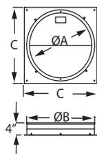
Use as a starter section for DuraTech. Bolts directly to fireplace outlet. Damper section allows chimney to be closed when fireplace is not in use. Includes chain and lintel hook.
