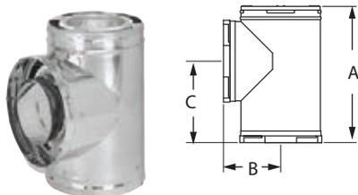
Use for through-the-wall chimney installations. The tee clean-out cap is removable for easy chimney cleaning or inspection. Wall Straps, a Wall Thimble, and a Tee Support must be installed with the Tee as directed. Tees have 1" insulating blanket. Ventilation air for chimney must be drawn from outdoors. (See installation instructions.)
