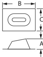
Use to weather proof the penetration of vent pipe through the roof. Storm Collar required. Select roof flashing based on pitch of roof. For pitches of 0/12 - 6/12. Made of galvalume.
