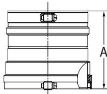
Use to connect 8" diameter PolyPro vent system to the Fulton EDR 2000 model appliance. No adapter connector and/or locking band required. Hose clamps on both ends.
