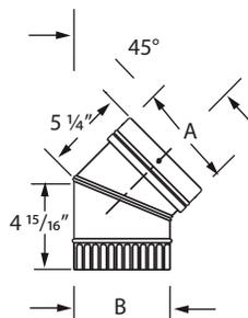
Use as a insert connector to DuraLiner. Features built-in fittings for easy connection to DuraLiner. Elbows are single-wall.
