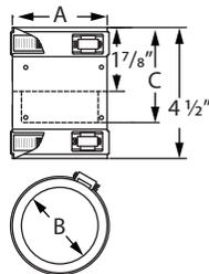
Use as a drip free connection between two sections of liner.
