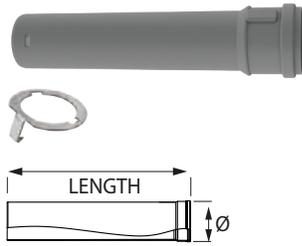
Use to vent condensing appliances. 2" (60mm) of overlap at the joint. Listed to ULC S636. Locking bands are required at all joint connections. Includes 1 Locking Band per each length .
