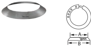
Required with DuraPlus flashing to create a weather proof penetration through the roof deck. Seal inner edge of the collar to the chimney pipe with non-hardening 500°F high-temperature sealant.
