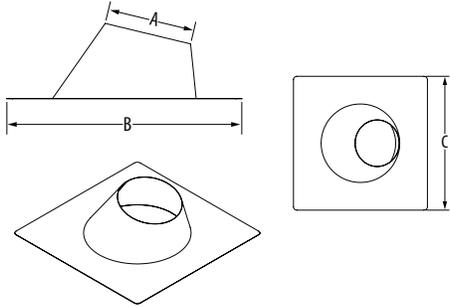
Use to to weather-proof the penetration of the galvanized outer jacket through the roof. Made of galvalume.
