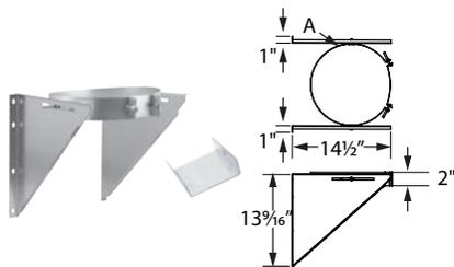
Supports up to 20' of DuraTech chimney. Can be installed above or below the tee. Adjustable base slides easily to provide between 2" and 6" of clearance to the wall. Can be used in place of tee support for chimneys under 20'. Or as an addition to tee support that goes beyond 50'.
