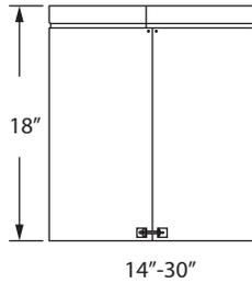
Use to add length to a straight length of Type B Gas Vent. 12" adds 3"-10" of length, 18" adds 10"-16" of length. Requires a 2" overlap.
