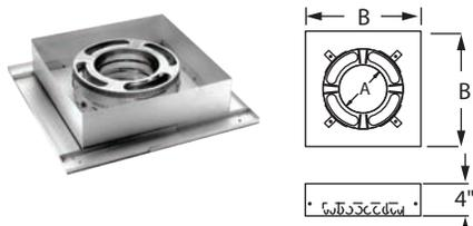
Supports chimney pipe and provides a positive connection between support box and chimney with a built-in twist-lock. Designed for installation in flat ceilings only. Supports up to 35' of DuraPlus chimney pipe. Use adapter to attach DVL or DuraBlack to the support box. A 2" wide trim collar is included. Not painted, but can be painted with high temperature paint. For adapters, see DVL and DuraBlack section.
