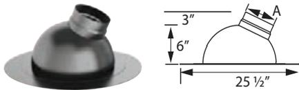
Use to weather proof penetration of vent through the roof. For concentric pipe. Made of aluminum. Adjusts from 0/12 to 5/12.
