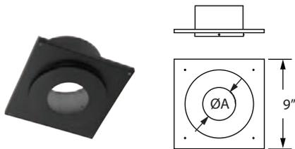
Required where vent passes through ceiling. Centers pipe to provide proper 1" clearance. Support Clamp included. Painted black.
