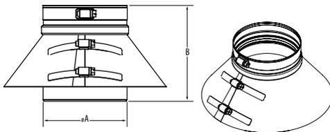
Use to vertically terminate a Double-Wall PolyPro system. Includes a AL29-4C stainless steel termination pipe with collar.
