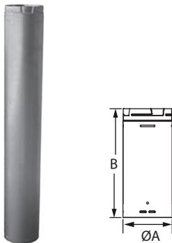
Use to reline masonry chimney with 0/0 clearance. Factory-insulated. Twist-lock fittings and pre-drilled hole (one screw required). UL Listed for zero clearance between masonry and combustibles, plus zero clearance between liner and masonry. 304 stainless steel inner and aluminized steel outer. Note: to calculate the installed length of 5", 6", and 8" DuraLiner pipe subtract 1 1/2" from each joint overlap of liner pipe sections.
