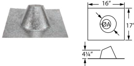
Use to weather proof the penetration of vent pipe through the roof. Storm Collar required. Select roof flashing based on pitch of roof. For pitches of 0/12 - 6/12. For steep roof pitches, refer to the Type B Gas Vent section.
