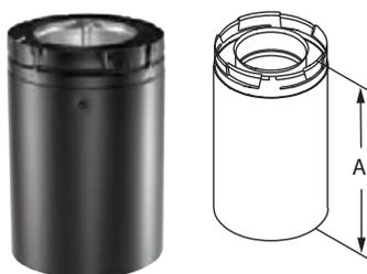
Use to add length to a straight length of DirectVent Pro. 8 1/2" pipe adds 3" - 7" of length, 16" pipe adds 3" - 14 1/2" of length, when used with rigid sections of pipe. Direct vent lengths feature a fully unitized, twist-lock construction. Use of sealant is optional, unless specified by the appliance manufacturer. Available in black or galvalume exterior (both feature laser-welded outer wall seams). Does not fit DirectVent GS pipe.
