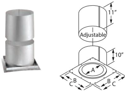
Use in ceiling/floor penetrations when a ceiling support is not used. Not required when passing through the roof. Fits on underside of ceiling and adjusts to cover framing.
