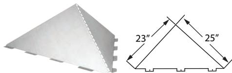
Three times thicker and stronger, allowing it to stand up against heavier snow loads. Bendable attachment flanges allow it to mount on any roof slope. Use to divert snow around chimney, vent and roof flashing. Constructed of paintable galvanized material. Ships flat for easy assembly. Works with 6", 7", 8", and 10".
