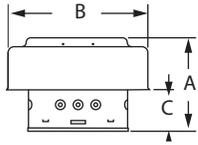
Required where pipe terminates above the roof line. Use for vertical installations only.
