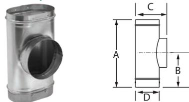
Provides connection between Masonry Wall Thimble, Wall Pass Through, or stove connector pipe to oval DuraLiner. Single-wall. May require additional insulation. Refer to DuraLiner installation instructions.
