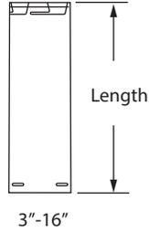
Use for venting listed natural gas or liquid propane Category I, draft hood appliances, or appliances that have been specifically tested and listed to use Type B Gas Vent. The appliances listed typically use Type B Gas Vent systems, but not always: Furnaces, Water Heaters, Boilers, Room Heaters, Decorative Gas Appliances, and Unit Heaters.
