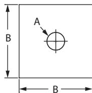
Use to close the top of a masonry chimney and to provide support for the liner.
