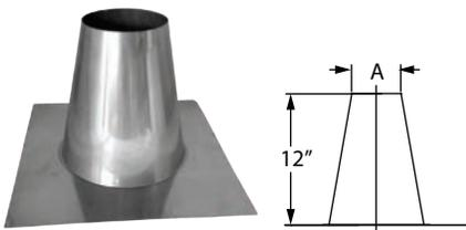
Use to create a weather-tight penetration where the vent pipe passes through a flat roof. Storm Collar required. When ordering Flashings for FasNSeal W2 product the flashing diameter and vent diameter are the same. ie. W2-3610 requires a FSVPF10.
