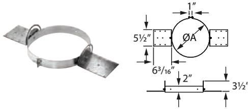
Use to help support weight of DuraChimney II. Supports a maximum of 25' of chimney. Use additional Supplementary Supports as needed.
