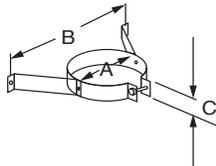
Designed for use on an interior or exterior wall, it serves to stabilize the chimney while providing the required clearance from the combustible surface. The use of wall bands at maximum intervals of 8' is recommended.
