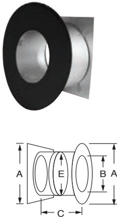
Designed to protect surrounding combustible materials when a chimney crosses through a wall horizontally, this shield can be adjusted from 7" to 12-1/2" to adapt to the thickness of the wall opening. A decorative plate painted in matte black provides an interior finish. Insulated to prevent cold air intrusion.
