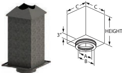
Use with flat, vaulted or cathedral ceilings where there is an attic space above. Supports up to 40' of DuraTech Chimney. The additional Insulation Collar now enables the support box to be qualified as an Attic Insulation Shield. The additional Attic Insulation Shield (DT-AIS) is not required with these support boxes.
