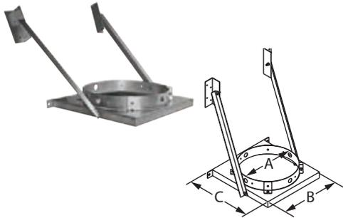
Use as wall support for chimney system. Supports up to 30' of DuraTech Chimney. Attaches to chimney pipe. Can be installed above or below the Tee. If installed below the Tee, a short section of pipe is required.
