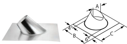
Use to weather proof the penetration of vent pipe through the roof. Storm Collar required. For roof pitches of 7/12 - 12/12. Made of galvalume.
