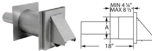
Use for horizontal through-the-wall terminations. Check installation instructions for restrictions on horizontal cap terminations, such as minimum distance from windows and doors. Accommodates wall thickness of 4 1/4" to 8 1/2". Damper prevents backdraft of cold air to appliance.
