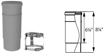
Use to add length to straight length of PolyPro pipe. Slips over any standard single-wall pipe length to form a telescoping pipe section. 4 1/2" (114mm) of adjustment. Adjustable pipe not available in 8" (200mm) diameter. Includes 1 Adapter Connector clamp.
