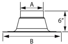
Use to weather-proof the penetration of vent pipe through the roof. For concentric pipe only.
