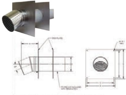
Use for through-the-wall horizontal terminations. Includes 23 degree termination elbow with integrated bird screen, inner and outer wall plates, and clamp for connecting to PolyPro pipe. No locking band is required. All components are stainless steel.
