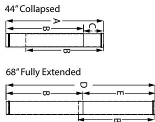
Use for a two-piece installation. Connects directly from stove to ceiling support box or finishing collar. Adjusts from 44" - 68". No cutting required.
