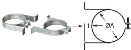
Use to provide support for offsets and horizontal runs. Recommended every 4' to support vertical vent.
