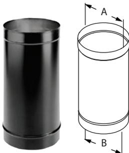
Use for a single-wall connector pipe. Requires 18" clearance to combustibles. Subtract 1 1/4" from length to calculate the installed length.
