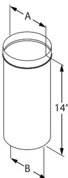
Use to adapt DuraBlack pipe to ceiling support box or finishing collar. Adds 3" - 13" of length to rigid pipe. Allows drip-free installation without cutting the pipe. Can be used in line to create a telescoping combination when used with a straight length of pipe. Requires screws.
