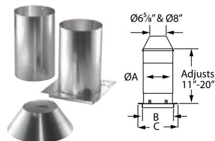
Required for installations that pass through an attic to prevent insulation and debris from accumulating near the vent. Provides 1" clearance to combustibles. Includes base w/tube, extension tube and collar.
