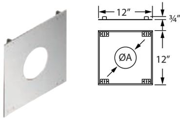
Use to protect exterior of structure from blower discharge in horizontal venting applications.
