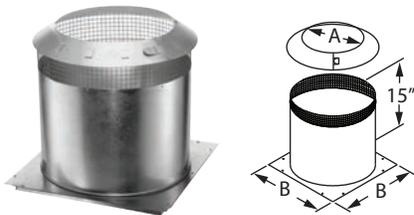
Use in installations that pass through an attic to prevent insulation and debris from accumulating near the chimney, unless chimney is enclosed through attic. Fits over Firestop Radiation Shield or a support box. Consists of two parts – a collar and a base. Mesh sleeve around top.
