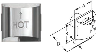
Use for horizontal through-the-wall termination. Check installation instructions for restrictions on horizontal cap terminations, such as minimum distance from windows and doors. Available in aluminum, stainless steel (S), and copper (C). Check with appliance manufacturer for approval. Patented.
