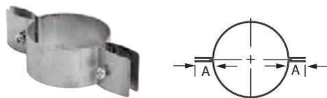
Use to support vertical and horizontal runs using threaded rod. Recommended every 10' on vertical runs and every 6' in horizontals. Use additional Support Clamps as needed.
