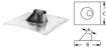
Use to weather proof the penetration of vent pipe through the roof. Storm Collar required. Select roof flashing based on pitch of roof. For pitches of 0/12 - 6/12. Made of galvalume.
