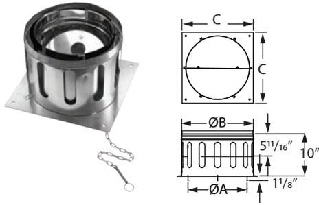
Use as a starter section for DuraChimney II. Bolts directly to fireplace outlet. Damper section allows chimney to be closed when fireplace is not in use. Includes chain and lintel hook.
