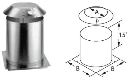
Required for installations that pass through an attic to prevent insulation and debris from accumulating near the chimney. Fits over Firestop Radiation Shield or a support box. Consists of two parts – a collar and a base.
