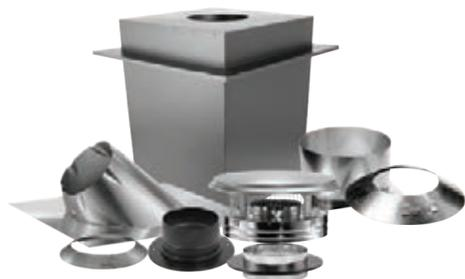
Kit includes: DVL and DuraBlack Chimney Adapter, Snap-Lock Adapter w/ Trim, 11" Square Ceiling Support Box with Trim, Adjustable Flashing 0/12-6/12, Chimney Cap, Storm Collar, and Attic Insulation Shield. Only available in 6" diameter. Pipe not included. Can be used for flat or vaulted ceiling installations.
