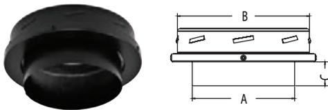
New integrated collar with adapter, fits into the female end of the chimney pipe to provide a decorative black finish. Use on chimney pipe that is suspended with the roof support system or on pipe that is passing through a wall thimble. Provides proper connection to DVL or DuraBlack. No other adapter is needed.
