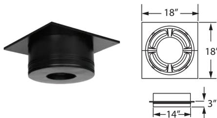
Supports chimney pipe and provides a positive connection between support box and chimney with a built-in twist-lock. Supports up to 35' of DuraPlus Chimney. Use adapter to attach DVL or DuraBlack to the support box. Painted black. Trim collar included. (For adapters see DVL and DuraBlack section.)
