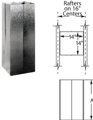
Use in installations where a 7" or 8" DuraVent chimney system passes through a roof opening with less than the normal 2" minimum clearance to roof trusses or rafters. Chimney pipe must be centered within Close Clearance Shield. (See installation instructions.)
