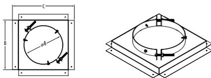
Use when penetrating floor levels with Double-Wall PolyPro and provide support at the ceiling level. Includes clamp that supports and prevents pipe sections from slipping down.
