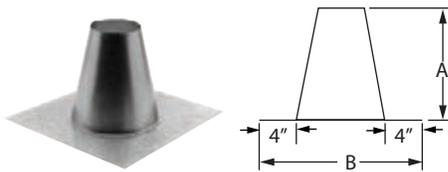
Use to weather proof the penetration of vent pipe through the roof. Storm Collar required. Select roof flashing based on pitch of roof. Use on flat roofs, chase enclosures, or masonry chimney. Made of galvalume.
