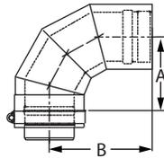
Use to go from horizontal to vertical runs or vertical to horizontal runs. Use to turn vent 90°.
