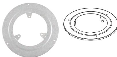
Conceals gap between pipe and wall cut out on the interior of a building. Bend tabs to secure. Neoprene ring reduces air infiltration where pipe slips through. Can only be used in a Gas Application.
