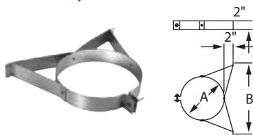
Use in interior or exterior installations to support and to stabilize the chimney while assuring a 2" clearance. Wall straps are required every 4' on exterior of building only.
