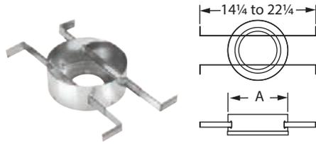
Use to support the Type B gas vent between 16" to 24" on-center joists or rafters. Use with a Draft Hood Connector to transition fitting between single-wall connector and Type B gas vent pipe sections. A Firestop Spacer is required.
