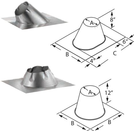
Use to weather proof the penetration of chimney pipe through the roof. Storm Collar required. Select roof flashing based on pitch of roof. For example, a 6/12 pitch has a vertical rise of 6" over a horizontal distance of 12". Made of galvalume.
