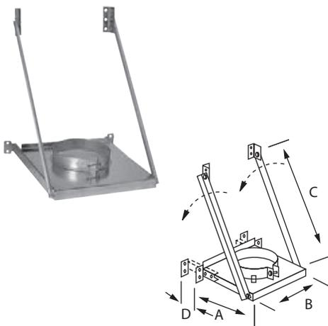
Supports the chimney at the base of the installation or along a wall or other vertical surface serving as an intermediate support. Also permits the tee to be installed above or below the support. It comes with a tightening collar locked around the chimney and secured by two self-tapping screws (included). The collar rests on a horizontal plate. When used as a base support, it lends itself to the addition of an insulated tee cap. Refer to chart for loadbearing capacity.
