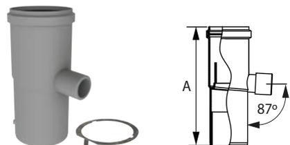
Use to remove corrosive condensates from within the vent system. 1-1/4" OD drain outlet. Includes 1 locking band. For 8" systems - use 8PPS-T with 8PPS-CD Tee Cap Drain.
