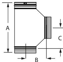
Use to transition from horizontal to vertical. Provides improved flue gas flow with angled gradual transitions. Can also be used as a manifold connection to gang boilers into a common vent.
