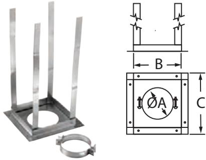
Use to support vent at ceiling level. Includes clamp that supports and prevents pipe sections from slipping down. Provides the mandatory 1" clearance to combustibles. Straps extend 16".
