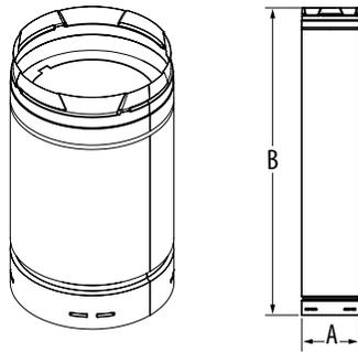
Galvanized outer jacket can be used as a conduit for single-wall PolyPro pipe. In exterior applications, provides protection from impact and UV light. Also provides some insulation value for use in colder climates. Can be field-painted if desired. Simple twist-lock assembly. To calculate installed length, subtract 1 1/2" for each joint. Includes internal metal support ring. PolyPro pipe sold separately.
