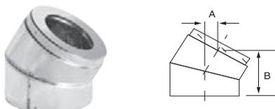
Allows the 30° offset of a chimney. Designed to bypass an obstacle, such as a joist. A maximum of two offsets (4 elbows) is allowed.
