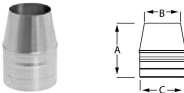
Use for vertical termination. Creates static back pressure to adjust harmonics. Venturi effect increases velocity of flue gases. Reduced opening provides for a smaller cross section to deter rain from entering the system. **Additional cones available in 1" or 2" reduction in diameter.**
