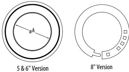
Used to maintain a weather tight, resistant seal between the galvanized outer jacket and flashing.
