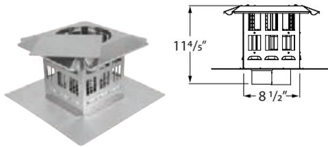
Use when installing a pellet insert into a multi-fuel pellet stove. This termination cap supplies both fresh air and vents exhaust. Lid pivots open for cleaning with three Removable screws and one rivet. Flex sold separately.
