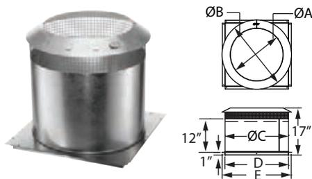
Use in all installations that pass through an attic to prevent insulation and debris from accumulating near the chimney, unless chimney is enclosed through attic. Consists of two parts – collar and base.
