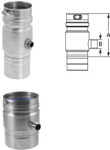
Use to properly manage corrosive condensates common with high efficiency gas appliances. For best results, install close to the appliance. Can be used horizontally, vertically, or any angle in between. The top photo shows the 3"-5" diameters with 5/8" straight tube; the bottom photo shows 6"-16" diameters with a 1" IPS Fitting.
