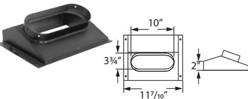
Use to connect inserts with 5" to 8" round flue collars to 8" Oval Flex Connectors. Made from 11 gauge carbon steel.
