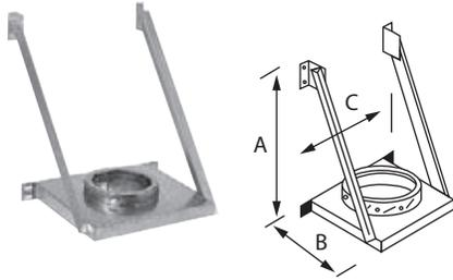
Supports the Tee and chimney at the base of the installation. First pipe length simply twist-locks into place on top of this support. Standard insulated tee cap that comes with the tee is fastened to the bottom side of this support's flue extension as per instructions.
