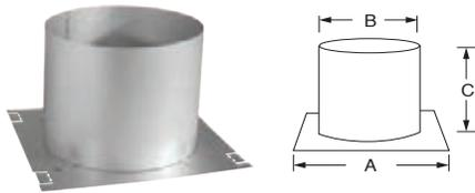
Protects combustible materials when the chimney passes through a floor or an intermediate ceiling. It ensures a 2" safety clearance between the chimney's outer casing and surrounding combustibles. When passing through a ceiling, it is to be installed from the underside of the ceiling. (Required in some jurisdictions in replacement of the firestop.)
