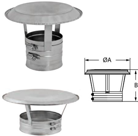
Use to support liner from the top and form a seal between the Storm Collar and the Top Plate. Top is removable for easy access to chimney cleaning. Top photo shows 3"-8" diameter style, bottom photo 9"-12" diameters.
