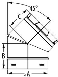
Galvanized outer jacket 45 degree elbow. Includes metal support ring. To calculate installed length, subtract 1 1/2" for each joint.
