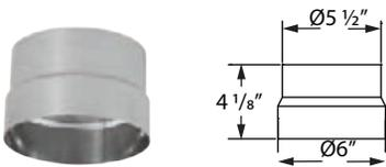
Use to connect 5 1/2" DuraFlex SS length to a 6" appliance. Check with the appliance manufacturer before reducing the vent size. May also be used to connect to stovepipe on a through masonry wall installations.
