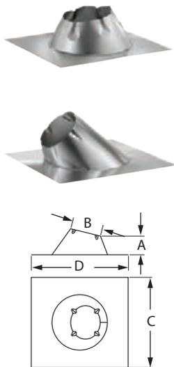
Use to weather proof the penetration of chimney pipe through the roof. Storm Collar required. Select roof flashing based on pitch of roof. For example, a 6/12 pitch has a vertical rise of 6" over a horizontal distance of 12". Made of galvalume.
