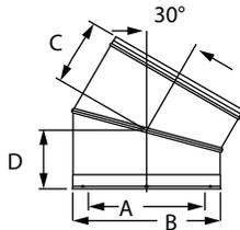
Use for offsets around obstructions such as rafters, ridgepoles, or joists. May have one pair of elbows if needed. Offsets greater than 30° are not permitted in accordance to UL 103 standards. Large diameters are restricted to one pair of elbows.
