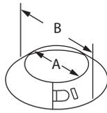
Required with DuraTech flashing to create a weather-proof penetration through the roof deck. Seal inner edge of the collar to the chimney pipe with non-hardening 500° F high-temperature sealant. Made of aluminum.
