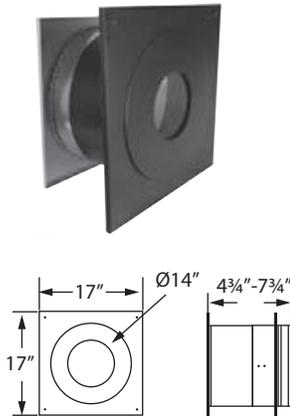
Adjusts from a minimum of 4 1/4" to a maximum of 7 1/4" wall thickness, and fits between standard wall studs. To accommodate thicker walls, the telescoping pieces can be extended up to 16" with a field-fabricated extension installed. Interior trim ring painted black. Must be installed with DuraPlus chimney pipe horizontally through the wall and extend a minimum of 2" into the room beyond the interior wall. For adapters, see DVL and DuraBlack section.
