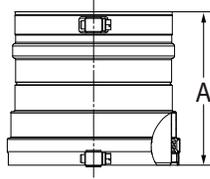
Use to connect 6" diameter PolyPro vent system to the Fulton EDR 750-1600 model appliance. No adapter connector and/or locking band required. Hose clamps on both ends.
