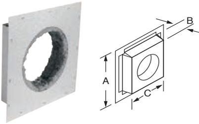
Designed for use with wood-burning stoves or fireplaces certified for use with chimneys, it should be used where the chimney passes through a ceiling or exterior opening where insulation is required. It must be used in combination with an attic radiation shield when passing through an attic. Recommended for use in cold regions.
