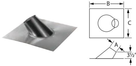
Use to weather proof the penetration of vent pipe through the roof. Storm Collar required. Select roof flashing based on pitch of roof. For pitches of 7/12 - 12/12. Made of galvalume.
