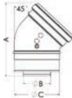
Use to vent condensing appliances. Offsets around obstructions as needed.
