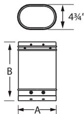
Use to reline masonry chimney with 0/0 clearance. Available in oval 6" and 8" diameters; 12", 24", 36", and 48" lengths. Factory-insulated. Built-in, pre-drilled fittings for riveting joints. 304 stainless steel inner and aluminized steel outer. Note: to calculate the installed length of 5", 6", and 8" DuraLiner pipe subtract 1 1/2" from each joint overlap of liner pipe sections.
