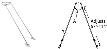
Extended roof bracket; provides additional support for the chimney when the chimney extends more than 5' beyond the roof; the legs will extend to handle varying roof slopes. New sandwich clamps allow legs to be extended to any length from 67" to 114". No drilling required.
