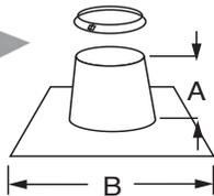
This component seals a chimney length when passing through a flat roof and comes complete with a storm collar.
