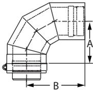
Use to transition from a vertical to a horizontal run. Facilitates a 2° pitch towards the condensate drain for good condensate management.
