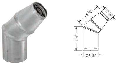
Use for horizontal terminations only. The Horizontal Cap can be turned at the gore to direct exhaust output. Designed to create a venturi effect to force exhaust out. Made of a laser-welded, super-ferritic stainless steel inner wall that is scientifically proven to resist corrosion from corn and other biofuels. Outer wall made of laser-welded stainless steel.
