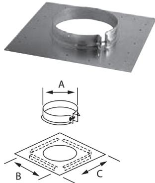
Use to support the chimney on a slab, floor, or joist and also acts as a firestop. It makes it possible to maintain a 2" clearance between the chimney's outer casing and combustible materials in its path. It includes a tightening collar that locks around the chimney and is secured by self-tapping screws (included). The collar rests on a horizontal plate screwed or nailed to the floor or slab. It can also serve as an intermediate support. Refer to chart for loadbearing capacity.
