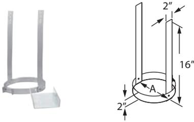
Use to prevent excessive weight on the elbows by supporting the weight of the chimney. Required to be installed between two elbows in offset installations. Multiple elbow straps may be required for offset installations. Refer to installation instructions.
