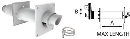
Use for concentric horizontal terminations. Includes white wall plate, 2 Locking Bands, white firestop, and co-linear adapter. White Termination with Bird Guard Screen. UV resistant. Inner plate is 8 5/8" (220mm) square, outer plate is 9 7/16" (240mm) square for all flue sizes.
