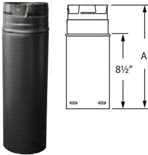
Use to add length to PelletVent Pro pipe. 12" pipe adds 3"-10" of length, 18" pipe adds 3"-16" of length, when used with rigid sections of pipe. Galvalume or painted black outer finish.
