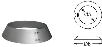
Required with DuraTech flashing to create a weather-proof penetration through the roof deck. Seal inner edge of the collar to the chimney pipe with non-hardening 500°F high-temperature sealant.
