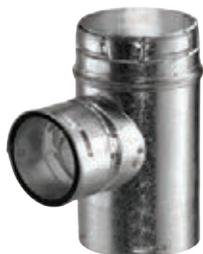
Attaches smaller pipe to branch and larger pipe to body. Use for a 90° offset or to combine connectors from two or more appliances into a common vent. Branch swivels for alignment.
