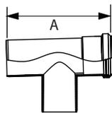
Use as a termination. Made of UV resistant polypropylene. Gasket not included. Includes 1 Locking Band. Bird Screen sold separately.
