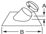
This part is required to accommodate sloped roof installations.
