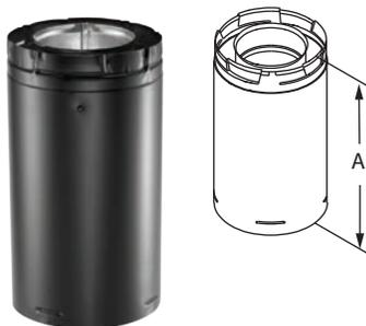
Designed for appliances tested and listed for direct vent. Features a fully unitized twist-lock construction in both 4" x 6 5/8" and 5" x 8" vent sizes. Use of sealant is optional, unless specified by the appliance manufacturer. To calculate install length, subtract 1 1/2" for each joint. No beads or hems. Black pipe lengths feature exterior laser-welded seams.
