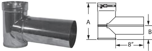
Use to attach to DuraFlex SS length with a fast connect band. Removable branch connects tee body with an internal fast connect band. 5 1/2" Tee has a 6" branch.
