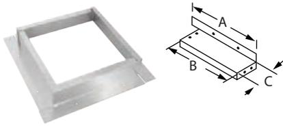
Use as a heat shield on structures with vinyl siding, or other temperature sensitive materials, to help prevent warping and or melting of the material. Use only on horizontal terminations and on any irregular surfaced siding (ie: ship lag siding, shake shingle siding) so cap is not imbedded in the siding. Kit includes 4-pieces; sized for Square Horizontal Cap only. Stainless steel (SS) and Copper (C) available.
