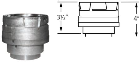
Use to attach to appliance outlet allowing for easy pipe connection. Allows connection of 4" vent to 3" appliance outlet. Seal adapter to appliance with high temperature sealant.
