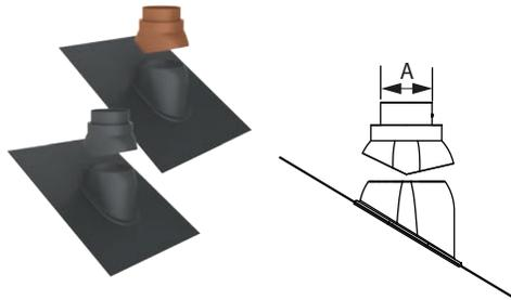
Use to weather proof penetration of vent through the roof. For concentric pipe. Made of polypropylene. Adjusts from 5/12 to 12/12. Black or terra-cotta. UV resistant.
