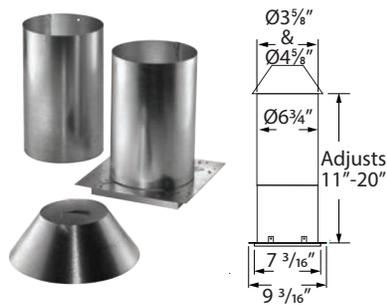
Required for installations that pass through an attic to prevent insulation and debris from accumulating near the vent. Provides 1" clearance to combustibles.
