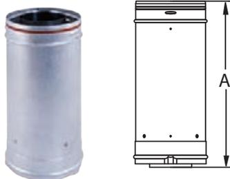
Features fully unitized, twist-lock construction in 3" diameters. It can be used in both vertical and horizontal installations. Stainless steel welded seam inner wall, combined with a galvalume weleded seam outer wall. Inner and outer are sealed with O-Ring gaskets. Galvalume or painted black outer finish. To calculate installed length, subtract 1 1/2" from each length of pipe.
