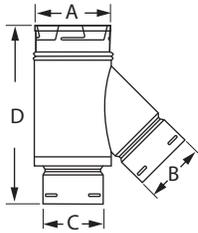
Use to combine connectors from two or more appliances into a common vent. Branch swivels for alignment. Swivel on male end. Additional sizes available through special order.
