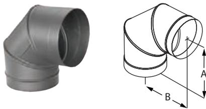
Offsets obstructions as needed or to orient the stovepipe horizontally for through the wall installation. Elbows angles are now adjustable. Adjustable elbows are manufactured drip free so creosote travels back to the stove as intended. Not recommended for rear exit appliances.
