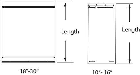
Type B Gas Vent systems may be used on other gas-burning appliances, when specified by appliance manufacturer. Type B Gas Vent is not used for Category II, III, or IV gas appliances, unless specified by appliance manufacturer.
