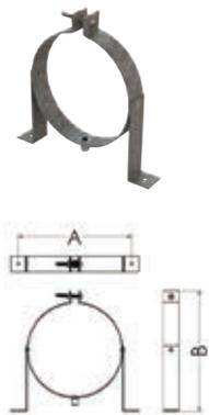
Use to support single-wall and concentric offsets and pipe used in vertical rise or horizontal runs as per installation instructions. Wall Strap legs can be rotated up to 360° for versatility. Accepts standard 1/4" all-thread. Available in galvanized or stainless steel metals. Note: Vent pipe must be supported at least every 10 feet (3m) vertically. Horizontal or sloped sections of vent pipe require a wall strap on each pipe section.
