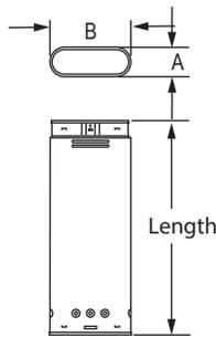
Use for venting listed natural gas or liquid propane Category I, draft hood appliances, or appliances that have been specifically tested and listed to use Type B Gas Vent. The appliances listed typically use Type B Gas Vent systems, but not always: Furnaces, Water Heaters, Boilers, Room Heaters, Decorative Gas Appliances, and Unit Heaters. Designed to be placed within 2" x 4" stud walls (4" and 5" oval pipe). 6" may only be placed in a 2" x 6" 16" O.C. stud space.
