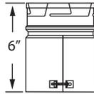
Use to connect DuraFlex AL to DuraVent Type B Gas Vent products.
