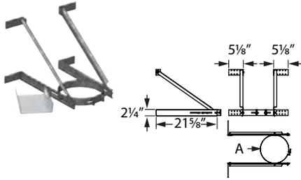
Use above the tee to provide support when bypassing obstructions or overhangs. Supports up to 20' of chimney. Tee Support is not necessary when using this support. For 5" diameter, it adjusts from 8 1/2" to 15 1/2". For 6" diameter, it adjusts from 8" to 15". For 7" diameter, it adjusts from 7 1/2" to 14 1/2". For 8" diameter, it adjusts from 7" to 14". Also available in Stainless Steel (SS).
