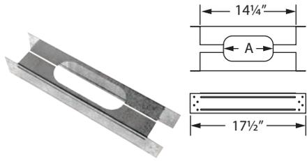
Use to center oval vent in a minimum 16" on-center stud space. Serves as a firestop at the ceiling level. Required in multi-story installations.
