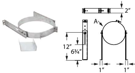
Stabilizes chimney while ensuring a minimum 2" clearance to combustibles. Can adjust out to 6" clearance if needed. One part covers 2 diameters (5" & 7" or 6" & 8").
