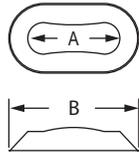
Use to maintain a weather tight resistant seal between the pipe and the flashing.
