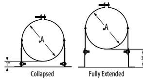
Use in interior or exterior installations to add lateral support to PolyPro DW Pipe. Adjusts to provide a 1"-3" clearance to combustibles and maintain proper slope. Additional clearance can be increased with optional PPS-WSMDW-EXT.
