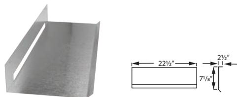
Required at top of chase enclosure or where chimney passes through the roof. Not required if chimney is unenclosed in the attic. Four plates (included) make up one shield.
