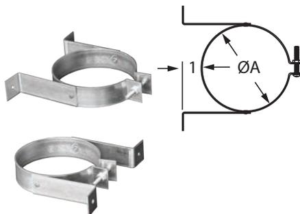
Use to provide support for offsets and horizontal runs. Recommended every 4' to support vertical common vent. Use also with DuraConnect or DuraConnect II. 10" Type B gas vent (11" OD) uses a 7" DuraPlus Chimney Wall Strap. Wall Strap legs can be rotated 360° to conceal screw.
