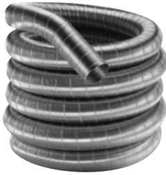
Use when relining masonry chimney for use with biofuel appliances. Made of super-ferritic stainless steel. Must be used with PelletVent Pro Male and Female Flex Adapters. Rigid pipe must be used when terminating system.
