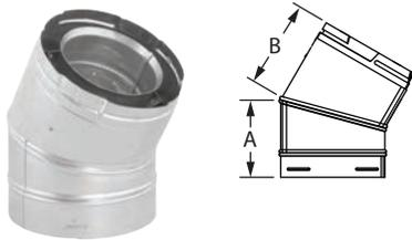
Use to offset obstructions as needed. Fully unitized, twist-lock construction. Elbows swivel, allowing the lock to remain fully engaged while aligning to the desired direction. The angle will remain fixed at 30°.
