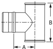
Use for standard and high-wind through-the-wall terminations. Check installation instructions for restrictions on horizontal terminations, such as minimum distance from windows and doors.
