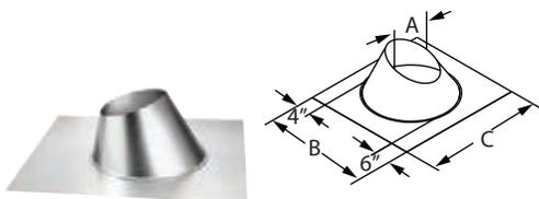
Use to weather proof the penetration of vent pipe through the roof. Storm Collar required. Select roof flashing based on pitch of roof. For pitches of 0/12 - 6/12. Made of galvalume.
