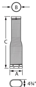
Use through damper and smoke shelf area. Use to connect from oval stove outlet to round DuraLiner. Use with DuraLiner Insulation Kit (ProMesh and ProFoil), where flex extends into clay liner, for zero clearance applications. Built from .016", 304 stainless steel, 4-ply construction.
