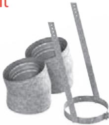
The 8" DuraChimney II Elbow Kits include 2 elbows and 1 elbow strap. Use to offset around obstructions such as rafters, ridepoles, or joists. Offsets greater than 30° is not allowed. Elbows are not adjustable.
