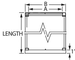
To calculate installed length of 10", 12", 14", 16", 18", 20", 22" or 24" DuraTech Chimney, subtract 1" from each joint overlap of chimney pipe. Important: Allow a minimum of 2" air space to combustibles when installing DuraTech Chimney.
