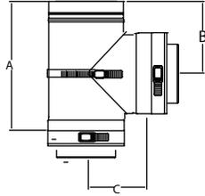
Use for a 90° offset, to combine connections from two or more appliances into a common vent or as a condensate management point when used in conjunction with drain fitting. All Standard Tees have completely welded inner walls.
