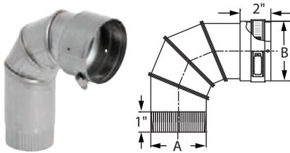
Use as a straight or up to 90° connection between liner and appliance flue collar.
