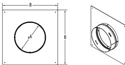
Used to trim interior wall penetration and transition from Double-Wall PolyPro (interior) to single wall pipe or Horizontal Termination (exterior). Includes built-in female twist-lock connection.
