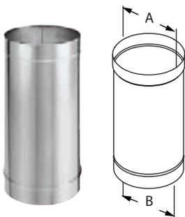
Use for a single-wall connector pipe. Requires 18" clearance to combustibles. Subtract 1 1/4" from the length to calculate the installed length.
