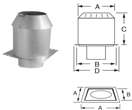
Also referred to as an insulation shield, it protects combustible materials when a chimney passes through an attic. It is imperative that it be installed overside from the attic. Its cone shape keeps insulation from seeping between the outer casing and the firestop. It also maintains a 2" clearance from combustible materials. Insulated to prevent cold air intrusion. Storm collar included.
