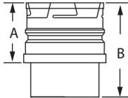
Use to connect appliance or single-wall connector to vent system.
