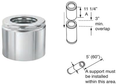
Used in combination with straight insulated lengths, the adjustable length makes it possible to fit a length perfectly. **IMPORTANT:** The adjustable length is not designed as a load-bearing component. Its vertical installation requires an appropriate support on the section above it to bear the weight of the remaining installation.
