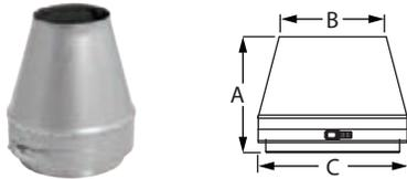
Use for vertical termination. Creates static back pressure to adjust harmonics. Venturi effect increases velocity of flue gases. Reduced opening provides for a smaller cross section to deter rain from entering the system. **Available in custom size combinations.**
