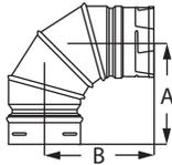
Offsets obstructions as needed. Elbows (3"-8") swivel 360° at base. 90° Elbow is adjustable from 0° to 90° in sizes 3"-10". Elbows must be supported when installed.
