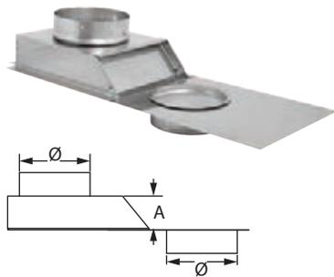
Use as a horizontally adjustable connector between a liner and top flue outlet of a heater. Adds up to 5" of offset.
