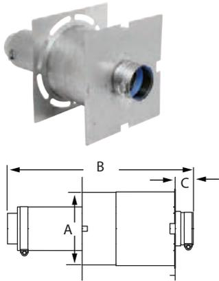
Use for through-the-wall termination. Fits between standard wall studs. 3"-5" diameters accommodates wall thickness of 4 1/4" to 8 1/2". 6"-16" diameters accommodate wall thickness of 5 3/4" to 11 1/2". AVL pipe allows for adjustability in length variance.
