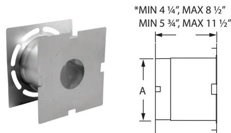
Use for through-the-wall termination. Fits between standard wall studs. 3"-5" diameters accommodates wall thickness of 4 1/4" to 8 1/2". 6"-16" diameters accommodate wall thickness of 5 3/4" to 11 1/2".
