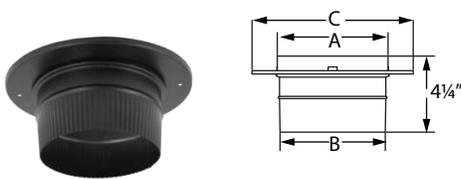
Connects into the ceiling support box or finishing collar and extends down to fit into stovepipe for a drip-free connection to a DuraTech, DuraPlus, DuraTech Premium, or DuraLiner Chimney system. Provides a strong mechanical connection. Adapter will work with all 6"-8" DuraPlus, 6"-8" DuraTech Premium, and 7"-8" DuraTech installations. Adapter will work with 5"-6" DuraTech Ceiling Support Box installations only.
