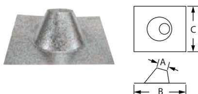
Use with metal or tile roofs. Available in sizes 3" and 4", in 0/12-6/12 (shown) and 7/12-12/12 styles. Made of dead soft aluminum.
