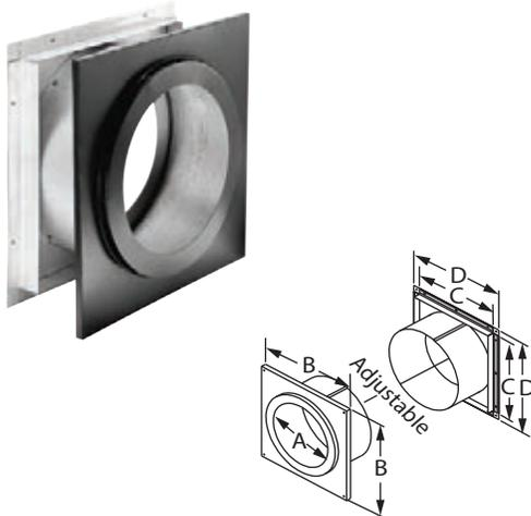
Adjusts from a minimum of 5 1/2" to a maximum of 9 1/2" wall thickness, and fits between standard wall studs. To accommodate thicker walls, the telescoping pieces can be extended up to 16" with a field-fabricated extension installed. Interior trim ring painted black. Must be installed with DuraTech chimney pipe horizontally through the wall and extend 6" into the room beyond the interior wall. (Black painted DuraTech is available). 6" and 8" stainless steel exterior trim available.
