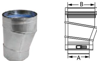
Use to transition to a larger diameter pipe. Adjusts the systems center point to offset from obstructions. Aids in reducing formation of condensates on horizontal runs. FasNSeal W2 has a 10" max change in diameter. **Additional sizes available up to a maximum of 10" diameter change.**
