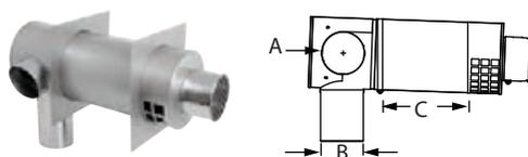
Use for through-the-wall termination with direct vent wall mounted gas appliances. Features a fixed right or left hand air intake snout and accommodates a maximum of 8" wall thickness. Check installation instructions for restrictions on horizontal termination, such as minimum distance from windows and doors.
