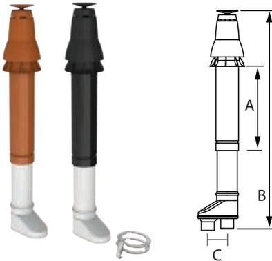
Use for concentric vertical terminations. Includes co-linear adapter and 2 Locking Bands. Black or terra-cotta cap. UV resistant. No storm collar required when installed with factory PolyPro flashing.
