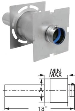
Use for through-the-wall termination. Fits between standard wall studs. 3"-5" diameters accommodates wall thickness of 4 1/4" to 8 1/2". 6"-16" diameters accommodate wall thickness of 5 3/4" to 11 1/2". AVL pipe allows for adjustability in length variance.
