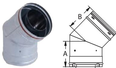
Offsets obstructions as needed. Allows for better condensate management and less back pressure. Sloped at 44° to direct condensate back to the appliance.
