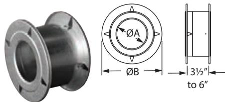
Use for through-the-wall system to provide clearances for vent from combustibles. Adjusts from 3 1/2" to 6" to accommodate various wall thicknesses. Larger diameter wall thimbles are field-fabricated. (See local codes for guidelines.)
