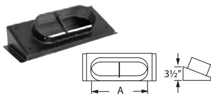
Use to connect inserts with rectangular flue outlets to Oval Flex Connectors. Top plate can point straight up or back towards the damper. Made from 11 gauge carbon steel.
