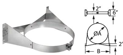
Use to support and to stabilize the chimney in interior or exterior installations to ensure a 2" clearance. Wall Straps are required every 8' on exterior of building only.
