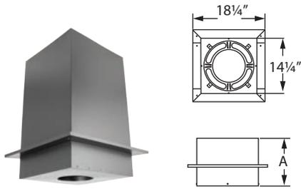
Use with flat, vaulted, or cathedral ceilings. Square Ceiling Support Box is painted black. Refer to Ceiling Pitch table to determine size of support box needed. Supports up to 35' of DuraPlus Chimney. Starter Section built-in. For adapters, see DVL and DuraBlack section. Trim included.
