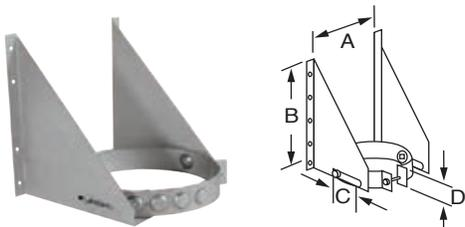
This part is designed to support the chimney on a vertical wall. The triangular plates allow a 2" to 4" lateral adjustment of the support to the vertical surface. This support can also be used as a wall support above the insulated tee. When used as a tee support, it lends itself to the addition of a Twist-Lock insulated tee cap.
