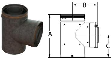
Use for a 90° offset. Tee has a 3x5 CVS connection for the branch. Includes removable clean out. Additional pipe cannot be used below the Tee Body.
