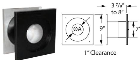
Use for through-the-wall installations. Fits between standard wall studs. Comes with an insulation ring to reduce air infiltration where the pipe slips through the thimble.
