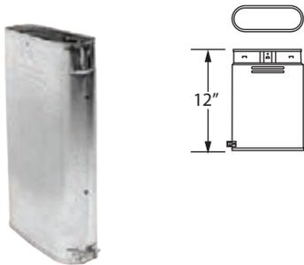
Use to add length to a straight length of Oval Type B Gas Vent Pipe. Adjusts from 4"-10". Requires a 2" overlap.
