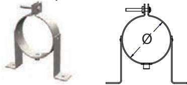
Use to support single-wall and concentric offsets and pipe used in vertical rise or horizontal runs as per installation instructions. Wall Strap legs can be rotated up to 360° for versatility. Accepts standard 1/4" all-thread. Available in galvanized or stainless steel metals. Note: Vent pipe must be supported at least every 10 feet (3m) vertically. Horizontal or sloped sections of vent pipe require a wall strap on each pipe section.
