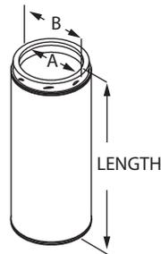
To calculate installed length of 5", 6", 7", or 8" DuraTech Chimney, subtract 1 1/4" from each joint overlap of chimney pipe. Allow a minimum of 2" air space to combustibles when installing DuraTech Chimney.
