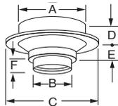
This part supports the chimney from a ceiling. Designed to connect to both double-wall and single-wall stove pipe, it is enhanced by a decorative black finish. Fits between standard 16"-on-center joists. Must be attached to a frame built from the joists. (Refer to chart on page 4 or 8 for loadbearing capacity and size of openings.) This finishing support has a removable trim collar for new construction installation.
