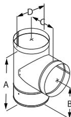
Use with rear exit appliances and appliances that require a barometric damper.
