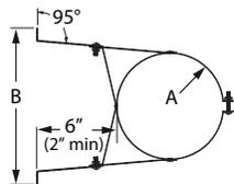
Use in interior or exterior installations to add lateral support to the chimney. Assures a 2" to 6" clearance to combustible walls. Required every 8'.
