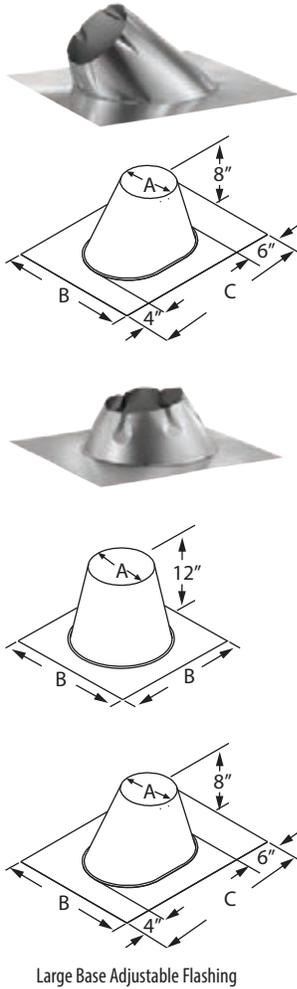
Use to weather proof the penetration of chimney pipe through the roof. Storm Collar required. Select roof flashing based on pitch of roof. For example, a 6/12 pitch has a vertical rise of 6" over a horizontal distance of 12". Made of galvalume. 6"-8" available with large base.
