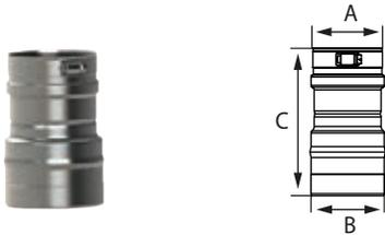
Use to connect PolyPro vent system to a standard stainless steel appliance outlet equipped with an integrated hose clamp and gasket. Must be used with Adapter Connector for flue gas, unless a clamp is supplied on the appliance outlet. Same O.D. as PVC.
