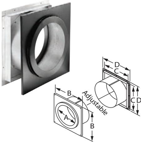
Use to provide clearance to combustibles. Adjusts from a minimum of 4" to a maximum of 10" wall thickness, and fits between standard wall studs. To accommodate thicker walls, the telescoping pieces can be extended up to 16" with a field-fabricated extension installed. Interior trim ring painted black. Must be installed with DuraTech chimney pipe horizontally through the wall and extend 6" into the room beyond the interior wall.
