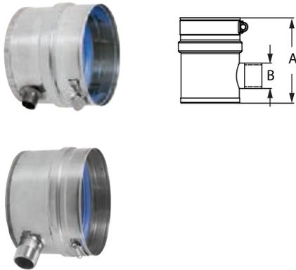
Use to manage condensates in horizontal runs. Optimal when ganging multiple appliances into a common vent. The top photo shows the 3"-5" diameters with 5/8" straight tube; the bottom photo shows 6"-16" diameters with a 1" IPS Fitting.
