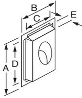
This part is to be used only with a wood-burning fireplace that have been certified for use with the chimney. It has been designed for use when the chimney passes through a wall at an angle.
