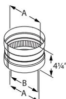
Use to adapt DuraBlack stovepipe to appliance flue outlets. Outer wall covers appliance flue outlet.
