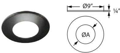
Reduces the center hole diameter in the Ceiling Support /Wall Thimble Cover to fit 3" or 4" pipe. Can be used as trim collar when penetrating a masonry chimney with PelletVent Pro. Painted black.
