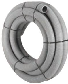
Use to line masonry chimneys that vent condensing appliances. Double-wall construction. Can be cut to precise length in the field. Available in 25, 35 or 50 foot lengths. 5" diameter flex comes in rolls of 98 feet only.
