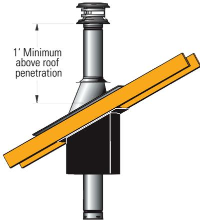
The following design recommendations are a general guideline to assist in the design and selection of venting components for your installation. Always follow DuraVent Installation instructions before installing your chimney system (found with the cap or support box). Installation instructions can be viewed online at [www.duravent.com](http://www.duravent.com), under Catalogs and Instructions.
